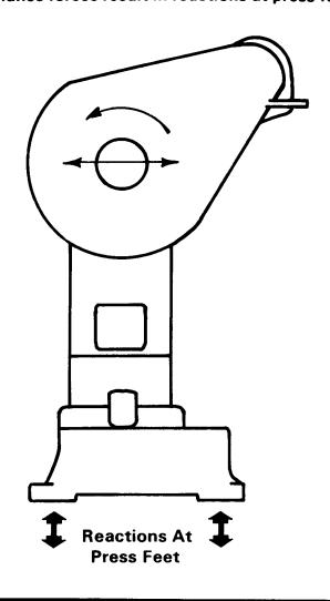
system. They act primarily along the direction of slide travel and tend to alternately lift the press free of the foundation and push the press into the foundation. In the cases of high speed machines, it is possible for the slide inertia force to exceed the dead weight of the press. It can then be seen that the press could be lifted free from the floor during a part of each stroke. This condition serves to estabish a limitation as to the available mounting approach for higher speed machines.
