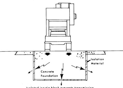
Isolated inertia block prevents transmission of shock/vibration to nearby areas
