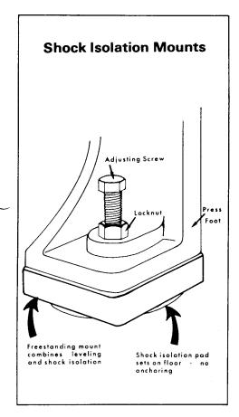
Shock isolation mounts can effectively serve installations where slide inertia forces are moderate (as in the case of a slow to medium speed machine or a high speed machine with a built-in dynamic balancer) and where sufficient support can be obtained from the existing floor. Here the condition of the floor and stiffness of the soil beneath the floor are primary considerations and must be carefully evaluated.
