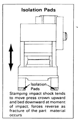
This approach is most often taken with smaller machines and involves the use of a resilient pad placed directly between the machine foot and the floor. The function of this pad is essentially the same as it would be in a shock isolating mount with the exception that the leveling capability is not present. When pads alone are used presses must be shimmed into level to assure proper alignments
